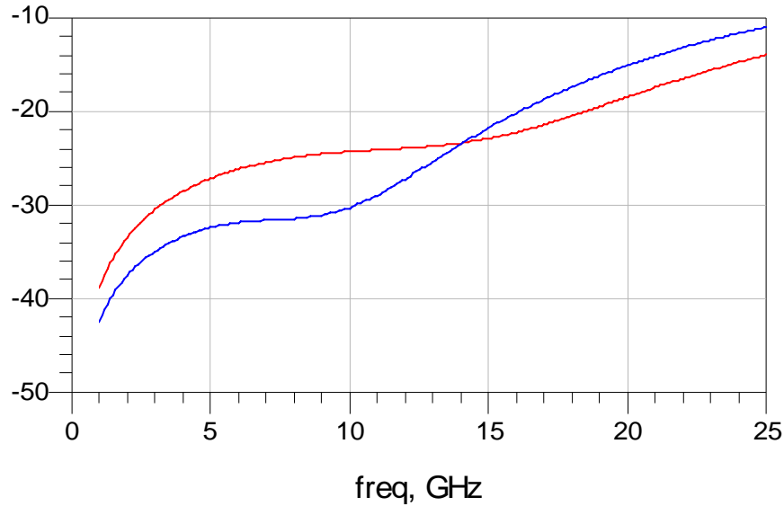
Figure 5. Two cases show return loss improvement for broad frequency (red) and specific frequency area (blue).
