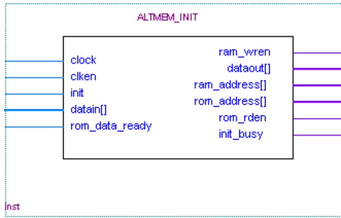
Figure 3–1. Input and Output Ports of the ALTMEM_INIT Megafunction
