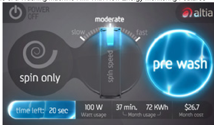
Figure 1. Example of a Washing Machine HMI With New Energy Monitoring Features
