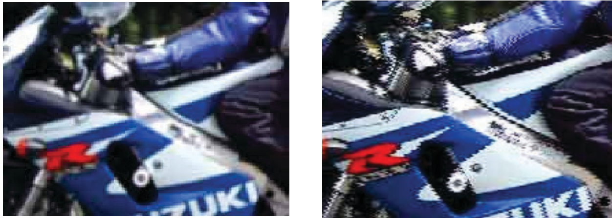
Figure 4. Differences Between Bob (left) and Weave (right) Deinterlacing
