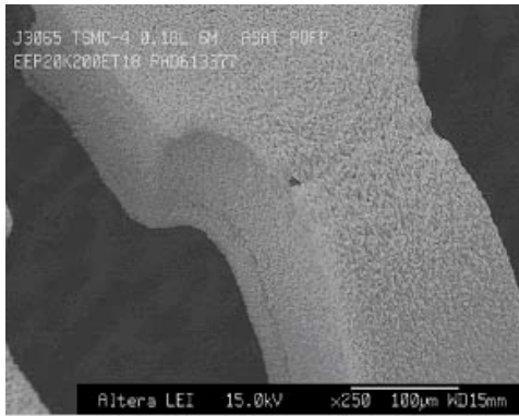
Figure 9. High Magnification View of a Matte Sn Finished Lead on a PQFP Device
