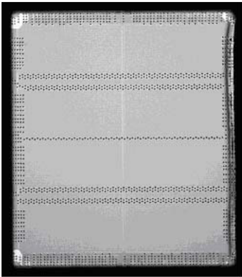
Figure 6. Die Corner Delamination Seen on Large Die Flip-chips with the Old Bill of Materials
