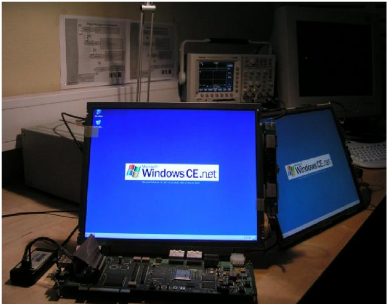
BADGE: Implemented on BitSim's High Speed FPGA Platform board, HIPPO.
