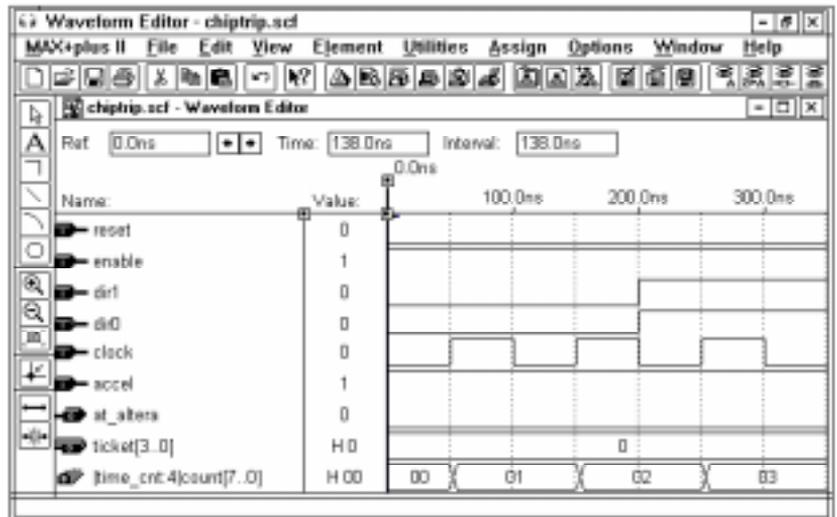
Waveform design entry is best suited for sequential and repeating functions. The Compiler's advanced waveform synthesis algorithms automatically generate logic from user-defined input and output waveforms that represent registered, combinatorial, and state machine logic. The Compiler automatically assigns state bits and state variables for state machines.
