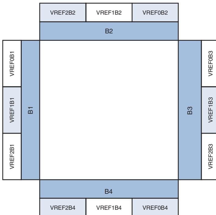
Additionally, each Cyclone I/O bank has its own  $V_{CCIO}$  pins. Any single I/O bank must have only one  $V_{CCIO}$  setting from among 1.5-V, 1.8-V, 2.5-V or 3.3-V. Although there can only be one  $V_{CCIO}$  voltage, Cyclone devices permit additional input signaling capabilities as shown in Table 8–4.
