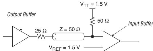
Cyclone devices support both input and output SSTL-3 Class I and II levels.
