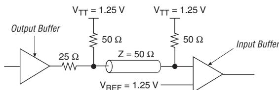
Cyclone devices support both input and output SSTL-2 Class I and II levels.
