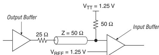
**Figure 8–4. SSTL-2 Class II Termination**
