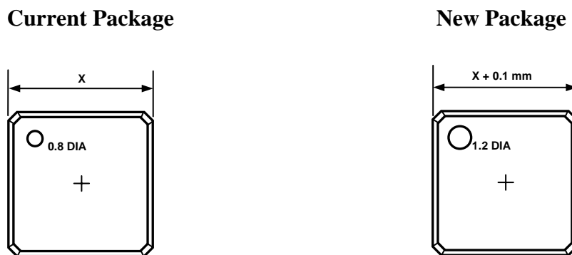
Figure 1 – Current and New TQFP 32 Package Dimensions
