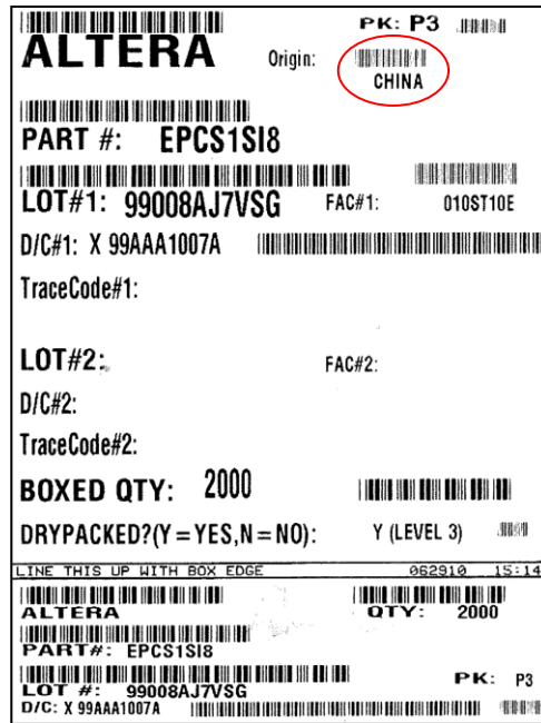
Figure 2. Assembly Site Location Identification on Box label
