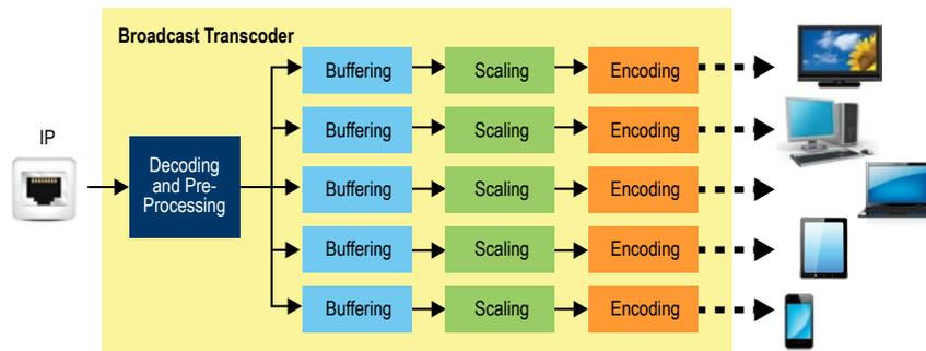
The various stages can be accomplished with many ASSPs/ASICs or integrated into fewer FPGAs with the same architecture. Either way, there are inefficiencies with this simple approach:
