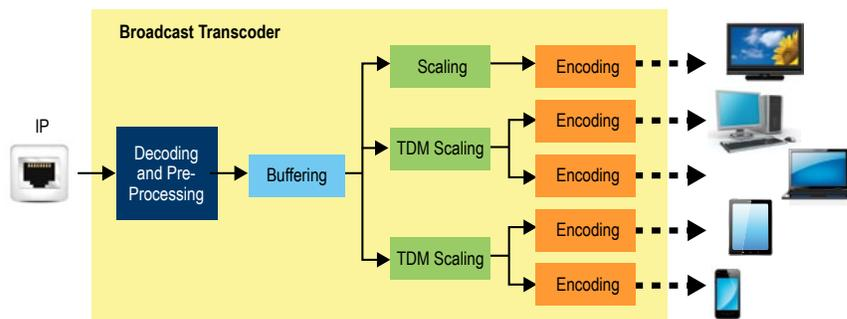
The number of outputs scaled with TDM depends on the ratio of input and output resolutions. The smaller the output resolutions, the more channels one TDM scaler can handle. If the encoder supports TDM as well, then the system can shrink further in size by removing the corresponding encoder instances.
