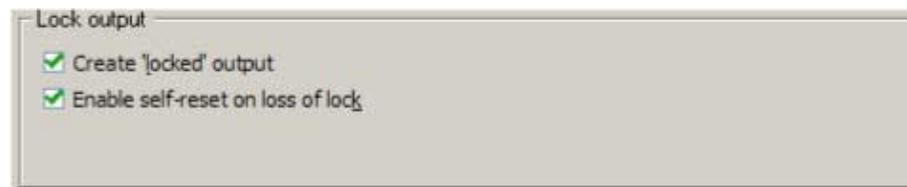
Turning on **Create 'locked' output** creates an output port named `locked` in the ALTPLL IP core.
