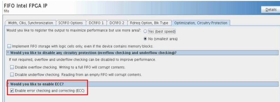
When you enable the ECC feature, a 2-bit wide error correction status port (`eccstatus[1:0]`) will be created in the generated FIFO entity. These status bits indicate whether the data that is read from the memory has an error in single-bit with correction, fatal error with no correction, or no error bit.
