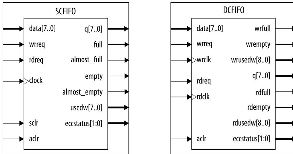
For the SCFIFO block, the read and write signals are synchronized to the same clock; for the DCFIFO block, the read and write signals are synchronized to the `rdclk` and `wrclk` clocks respectively. The prefixes `wr` and `rd` represent the signals that are synchronized by the `wrclk` and `rdclk` clocks respectively.
