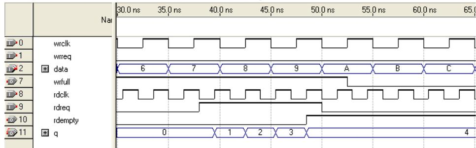
The required functional timing for the DCFIFO as described previously is also applied to the SCFIFO. The difference between the two modes is that for the SCFIFO, the wrreq signal must meet the functional timing requirement based on the full signal and the rdreq signal must meet the functional timing requirement based on the empty signal.
