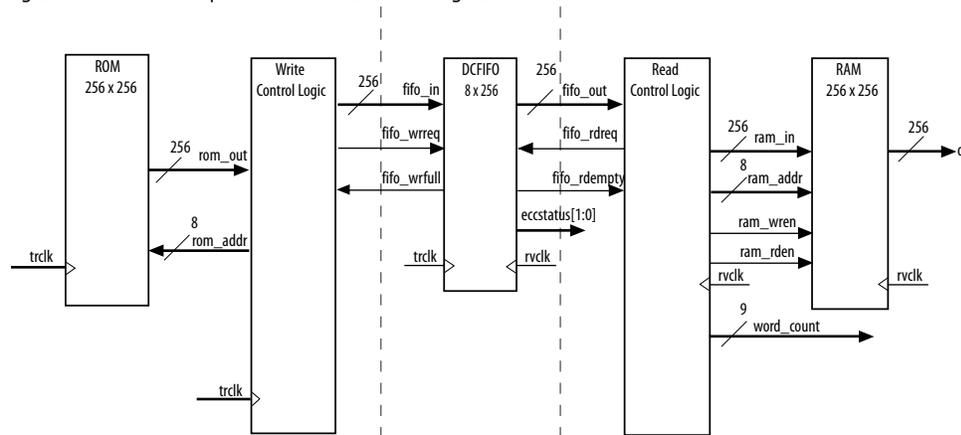
**Note:** The DCFIFO functions are with ECC feature enabled and implemented using M20K.
