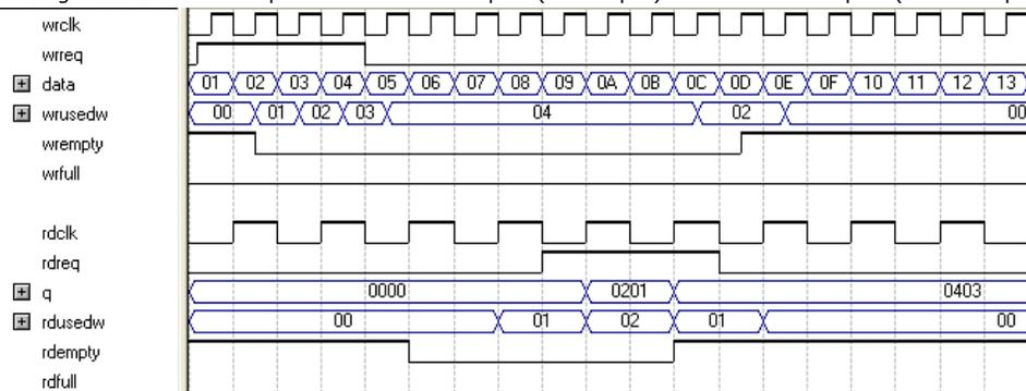
In this example, the read port is operating at half the frequency of the write port. Writing four 8-bit words to the FIFO buffer increases the `wrusedw` flag to four and the `rusedw` flag to two. Two 16-bit read operations empty the FIFO. The first and second 8-bit word written are equivalent to the LSB and MSB of the 16-bit output words, respectively. The `rdempty` signal stays asserted until enough words are written on the narrow write port to fill an entire word on the wide read port.
