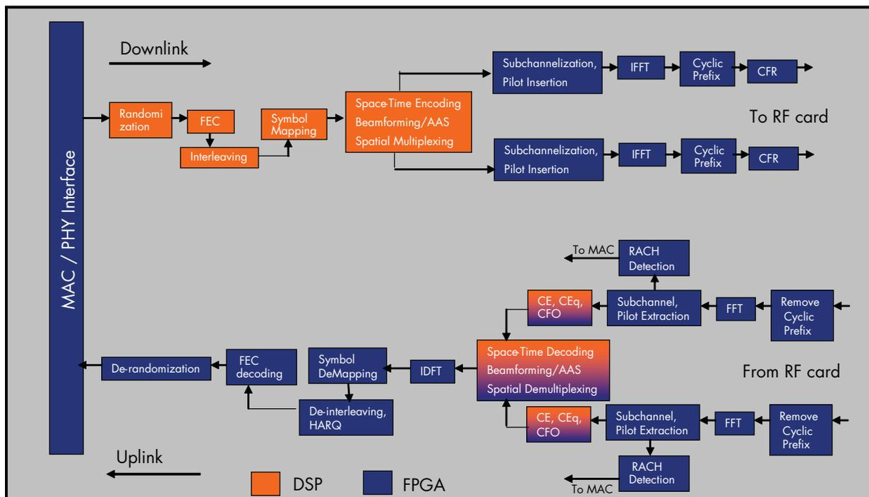
By incorporating advanced multiple antenna technologies, the throughput offered by such systems is expected to be over 100 Mbps. The baseband PHY functionality can be broadly categorized into bit-level processing and symbol-level processing functions. The following section covers these functions and how FPGAs are used to complement DSP blocks for implementing both bit-level and symbol-level functions.
