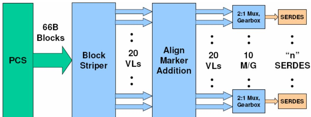
Figure 8 shows the receive path for the 100G PCS block. The receive channel demultiplexes the data from 10 (where  $n=10$ ) electrical lanes to 20 VLs. The receive channel deskews and aligns the VLs to rebuild the 66B data stream. Each VL on the receive path has its own dedicated FIFO buffer, the overall depth of which determines the skew tolerance limit of the design. For example, a FIFO buffer that is two 64-bit words deep will tolerate a 128-bit skew.
