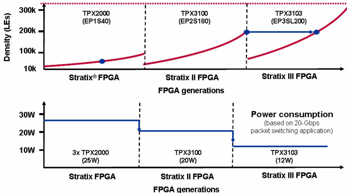
By moving from Stratix to Stratix II FPGAs, TPACK increased the capacity of the Carrier Packet Engine from 6 Gbps (TPX2000) to 20 Gbps (TPX3100), while decreasing the relative power-per-Gbps switching capacity. However, by porting this solution from Stratix II to Stratix III FPGAs (TPX3103), they reduced power consumption by as much as 40 percent.
