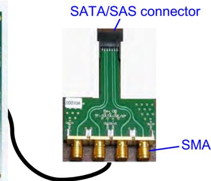
**Figure 6. Stratix IV GX FPGA Development Kit with SATA HSMC Daughter Card**
