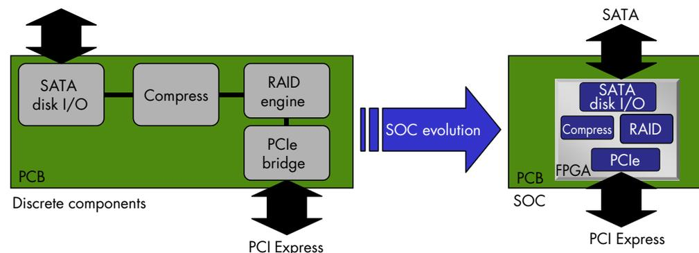
The FPGA offers an excellent platform on which to integrate many discrete ASIC or ASSP functions into a single chip solution. Now that Altera FPGAs support SAS and SATA natively with the integrated transceivers, it is possible to leverage the integration option for storage applications.
