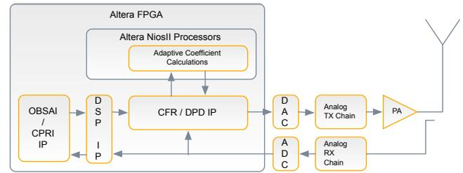
Figure 4: FPGA-Based Combined CFR/DPD Architecture.
