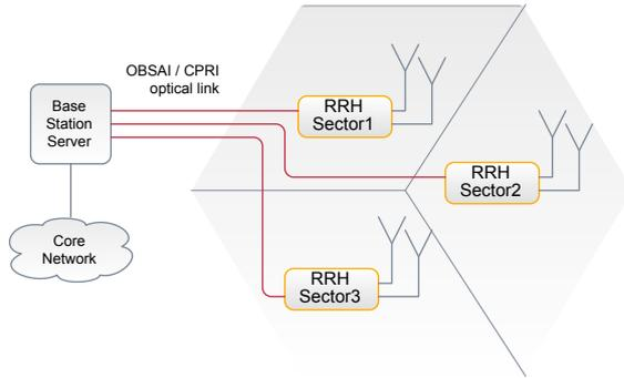
Figure 2: Three-Sector Wireless Call using RRH.
