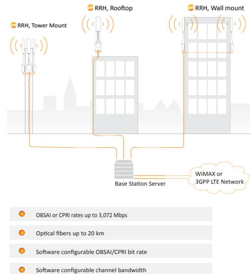
Figure 1: Distributed Wireless Base Station system.
