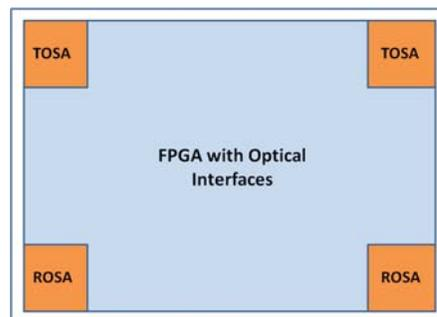
Designers can replace chip-to-module link systems with an optical interface FPGA to capture significant power, resource, and cost reductions, as well as an increase in port density, as illustrated in Figure 8. This is possible because Altera's advanced and power efficient transceiver has best-in-class clock generation and clock recovery, signaling conditioning and equalization, and built-in test and measurement via ODI.
