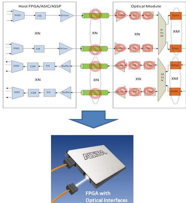
Figure 9 shows a generic application that includes an optical interface to the FPGA. Designers can use an FPGA with optical interface for an optical backplane, board-to-board, rack-to-rack, and system-to-system interconnect, with reach length up to 100 m at 10 Gbps line-rate. The maximum data rate for channel depends on the FPGA transceiver data rate, and is currently at 28 Gbps on the 28-nm process node.
