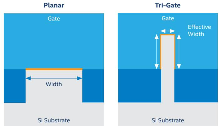
Figure 1. Effective Channel Widths of Planar and Tri-Gate Transistor Structures
