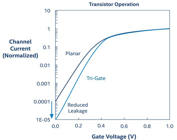
Figure 2. Tri-Gate Transistor Structures Provide Steeper Voltage Curves
