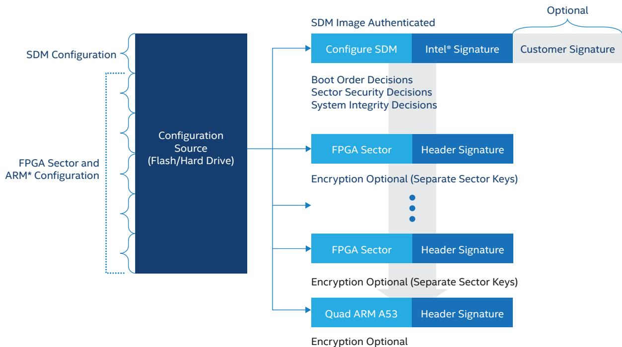
Figure 3. SDM for Intel Stratix 10 Devices Configures First, Followed by User-Designated Configuration Order
